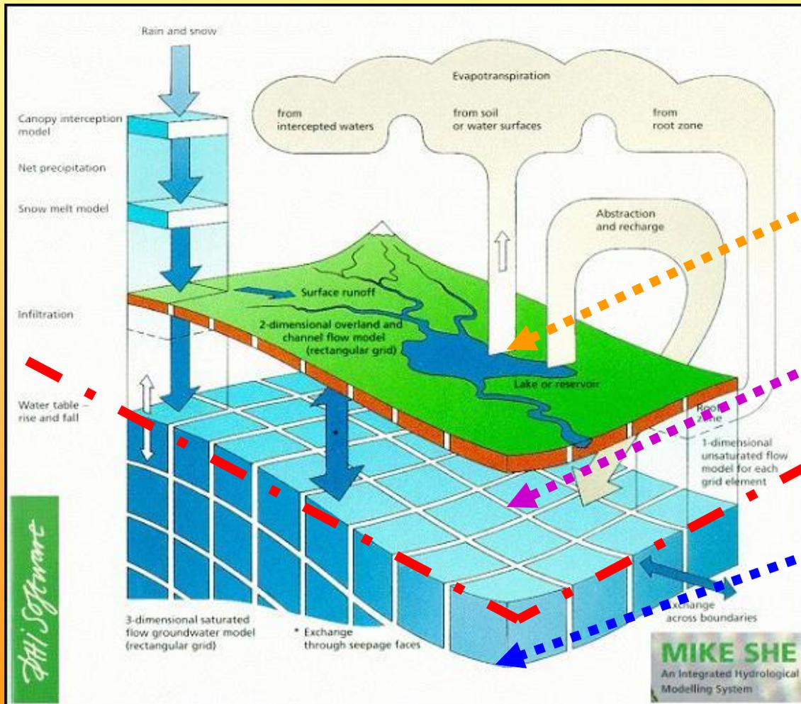
River network flow model (coupled with Rainfall-Runoff model)
